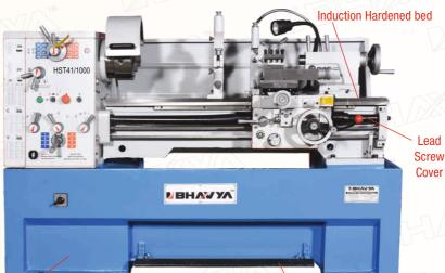
One Piece Solid Cast Iron Machine Base
