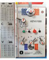
Speed & Feed Control Box with Metric, Imperial, DP & Module Thread Range
